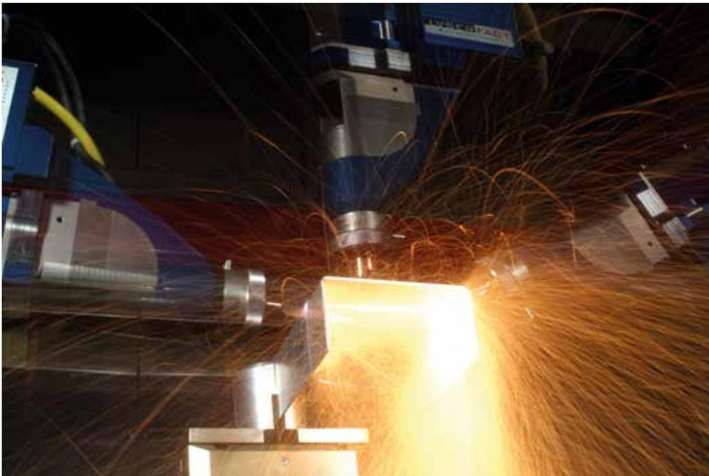
Processing methods using light: The laser combi-head is used for cutting and welding steel, as well as for additive manufacturing. The hybrid laser beam source consists of a diode laser for heat treatment and a fibre laser for cutting.
