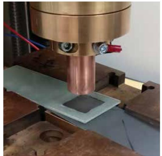
Welding an inserted hybrid test piece on a capacitor discharge welding system.
