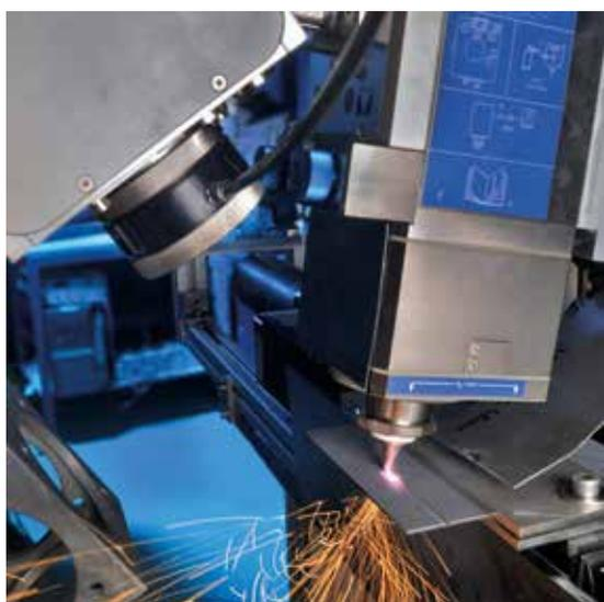
Laser cutting with tracking heat treatment laser. Local heat treatment can improve the crash properties of components by imprinting softer zones.
