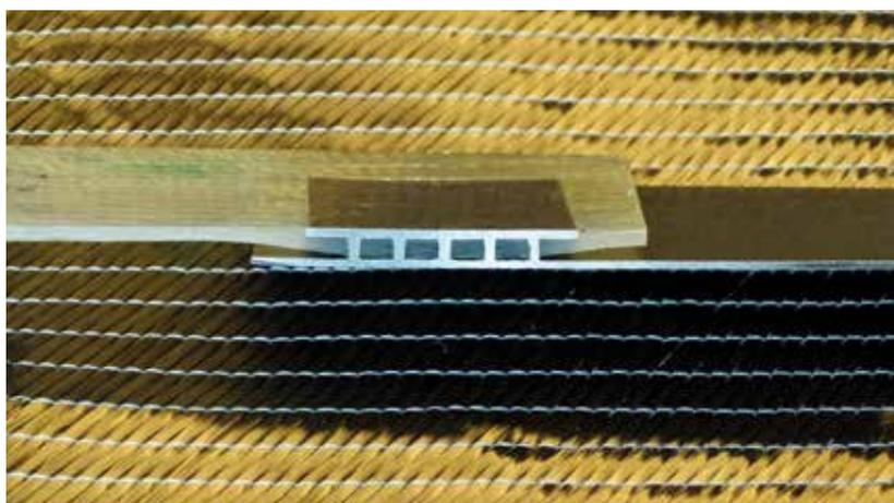
A finished welded hybrid test piece can be seen in cross-section.
