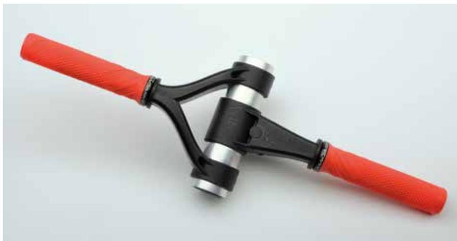
Compared to a hybrid component based on sheet steel, the hollow profile hybrid demonstrator has much greater dimensional stability, with better torsion stiffness and torsion strength.
