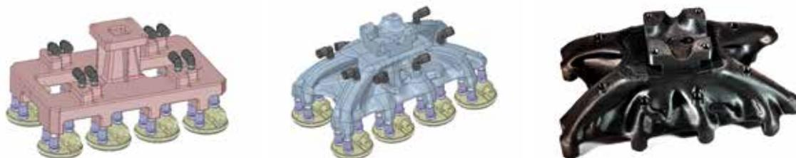
Left to right: traditional design, topology-optimised design, and a gripper produced using additive manufacturing.
