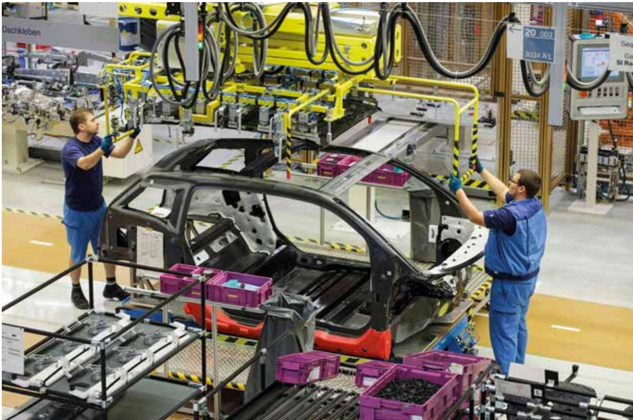
Hybrid construction methods are used for vehicle bodywork. Electric mobility is a driver of lightweight design. Steel is increasingly combined with other materials such as fibre-reinforced polymers.
